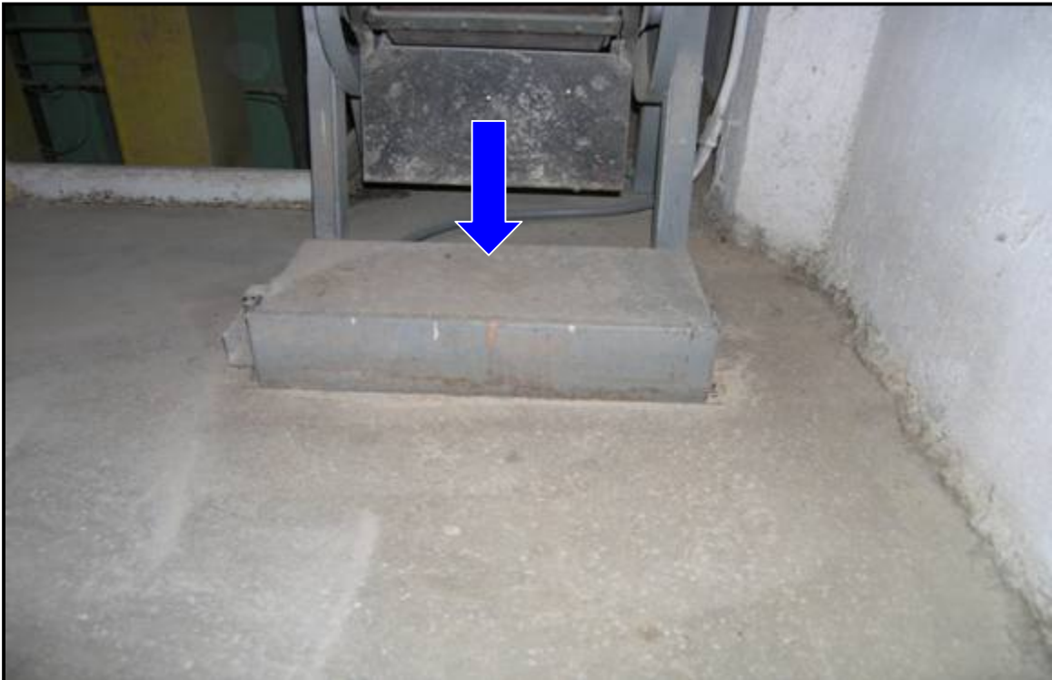
Emergency pads at the bottom will shut the belt off if an employee or object touches it.
